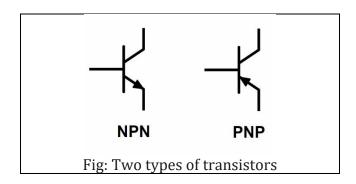
In the lab we will use NPN transistor (BD135). The transistor has three pins labeled as emitter, base and collector as shown in the following figure.
